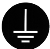
Connect ground wire
