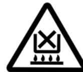
Caution for no liquid heating!
